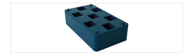
The K-Block 45C series has the same properties and functions as K-Block 45, but is simply in color-coded thicknesses. With its 45 mm, K-Block 45C is designed to accurately fit the width of rafters and other planed 2" wood, but is also used for distance adjustment and leveling of medium-heavy tasks such as doors and windows. The countersunk screw holes provide secure mounting.
